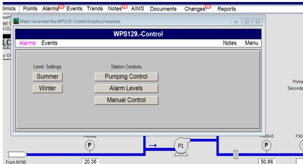
Figure 7: Remote Controlled Pump Station- Different Controls
