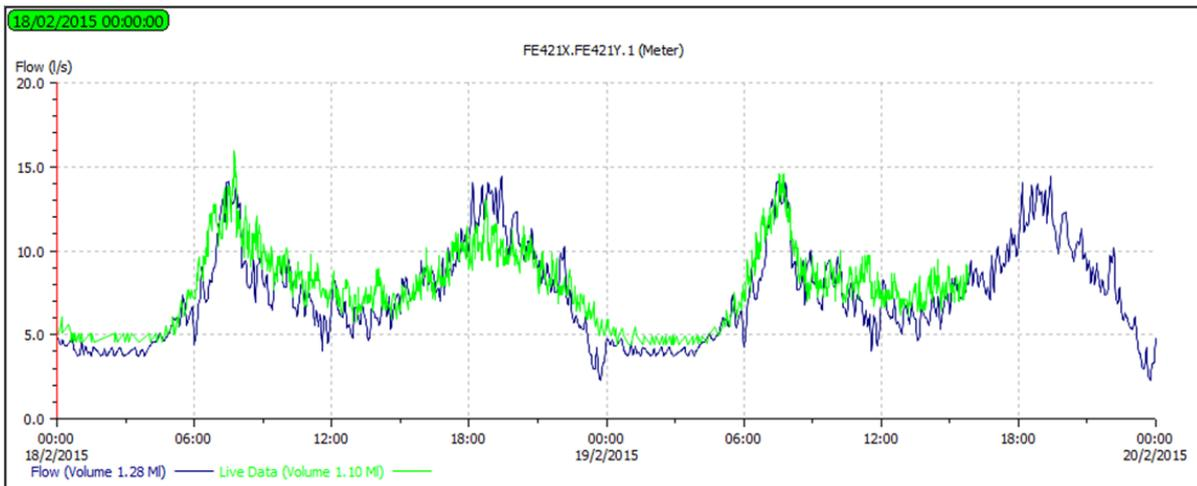
Figure 3: Model Prediction Vs Actual Flow (Verification Point)
