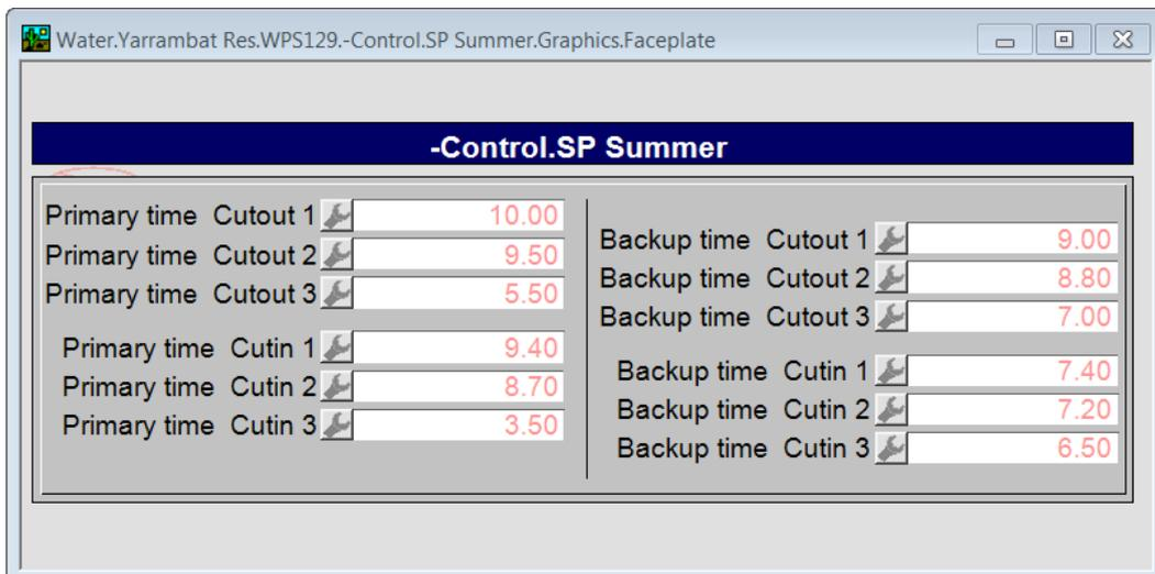
Figure 8: Remote Controlled Pump Station- Summer Controls
