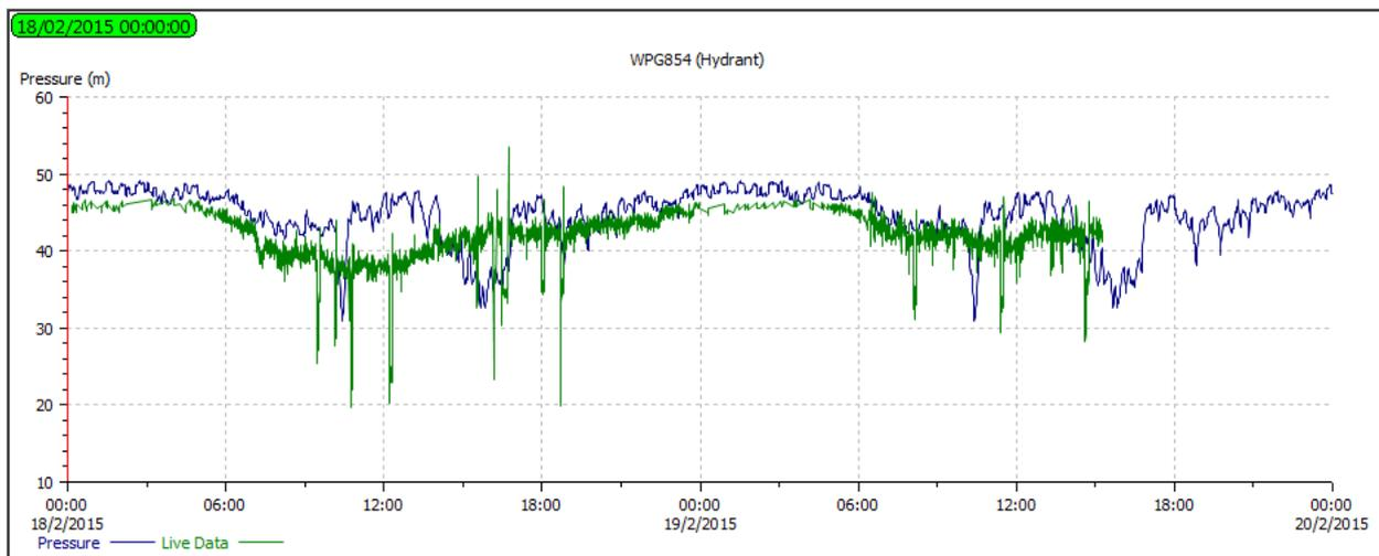
Figure 4: Model Prediction Vs Actual Pressure (Verification Point)
