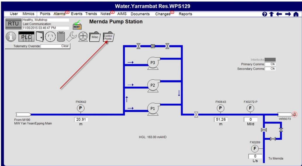
Figure 6: Remote Controlled Pump Station- SCADA Overview
