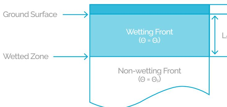
Figure 2: Two zone representation of the Green Ampt infiltration model (EPA website)
